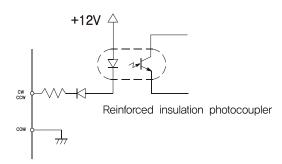
■ Example of input circuit connection
