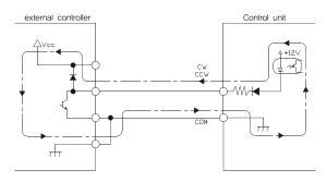
When you connect like the diagram above, if you turn the control unit power on first or if you turn the controller off while control unit is on, then the electricity flows and motor rotates.
