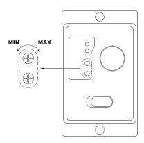
If you turn it clockwise, the time gets longer When you are changing the setting, use accurate cross screwdriver. In factory condition, it is set at the shortest time possible.
